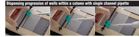
A similar set of detents on the shorter index bar provides the same alignment for the single-well isolator as the operator moves it down the column from well to well.
