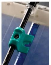
Well Mark can accommodate most plate variations through small, user adjustments to the device. The Well Mark has a sloped entrance to the column slot for easier single or multichannel pipette access and for accommodating raised features of some multi-well plates.
