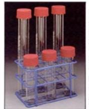
There are two models of the oven available, the H010 which holds two sizes of borosilicate glass bottles (35 x 300mm and 35 x 150mm) and the HO4 which holds four large size acrylic bottles. A tube rack to hold six of either glass bottles is useful for safe storage of tubes and for probe and buffer wash additions. The epoxy covered rack
