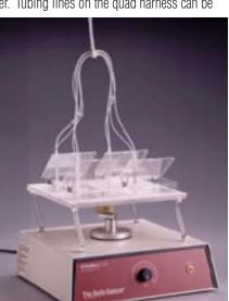
**Quad Harness** A guad harness with dispensing/aspirating bits for simultaneous processing
