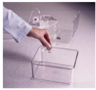
The dispensing/aspirating tube bits are designed to work with containers already in use in your lab. A stainless steel clip attaches the dispensing/aspirating bits to the side of the container. A nylon thumbscrew loosens to allow adjustment of the bits up or down to work with different container depths.
