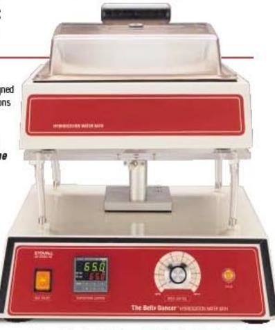
The combination Belly Dancer/Hybridization Water Bath unit consists of the bath along with a Belly Dancer modified to contain the temperature controls within the case.
