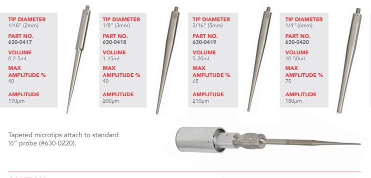
**CAUTION:** Do not exceed the maximum amplitude limits. Operating above the limit may cause the microtip to fracture. Do not use a tapered microtip with a coupler.
